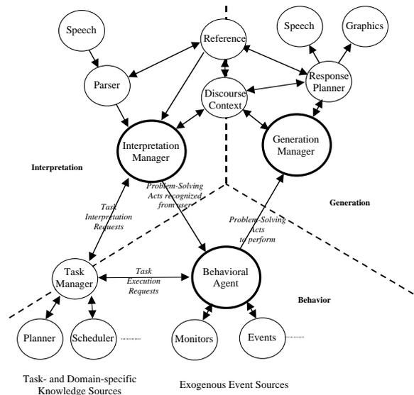
Figure 3: TRIPS collaborative system architecture (from [1])
